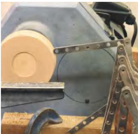
▲ Pic.7 This is one of my copying fingers set up on the diameter of the base. When the right amount of timber is cut away, then the finger falls down
